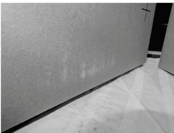
Fig. 10 Abrasion damage caused to test freight (Vibration condition C4)
