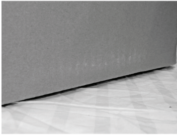
Fig. 9 Abrasion damage caused to test freight (Vibration condition C1)
