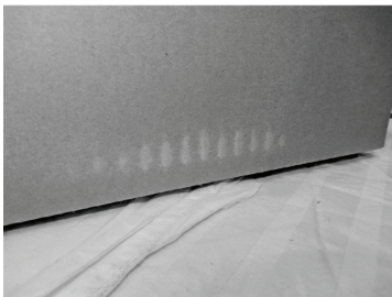
Fig. 11 Abrasion damage caused to test freight (Vibration condition C5)
