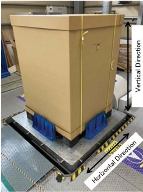
Fig.6 Vibration Test Scenery
