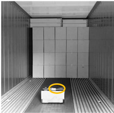
Fig. 7 A condition of the partition and the placement of the thermometer (Circle symbol) {The partition for the experiment patterns of (-6, 8), (-11, 8), (-21, 8) in Table 1}
