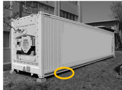
Fig. 4 A 40feet reefer container utilized for the experiment (The circle symbol is the placement of a thermometer.)
