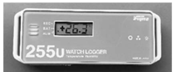
Fig. 5 A thermometer utilized for the experiment (WATCH LOGGER, KT-255U, Fujita Electric Works, Ltd, 2018)
