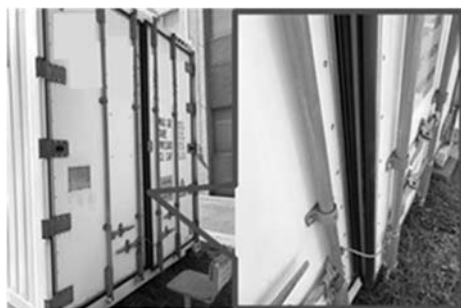
Fig. 3 The minimum opening onto a door of container when unlocked (approximately 3cm)
