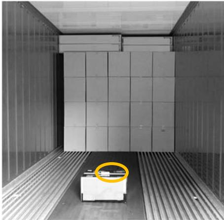
Fig. 7 A condition of the partition and the placement of the thermometer (Circle symbol)
