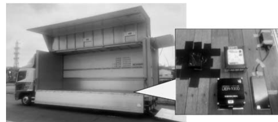
Fig.3 Shock and Vibration Measurement on Cargo Space of Truck
