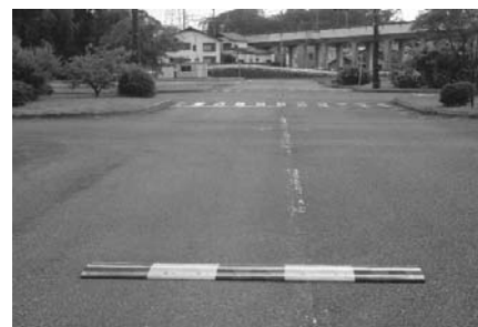
Fig.4 Bump of Truck Running Test
