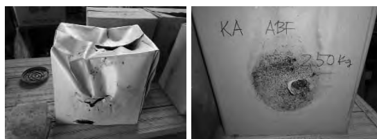
Fig7 Appearance of broken compost after experiment. (left: moisture proof 220 BF; right: K210 ABF)
