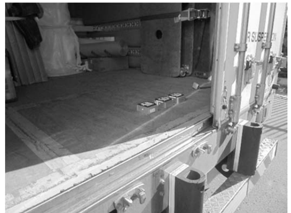
Fig.2 Acceleration data loggers on the loading platform of the truck.
