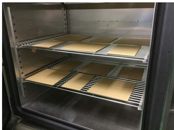
Fig.4 Setting Corrugated Sheets in Air Conditional Chamber
