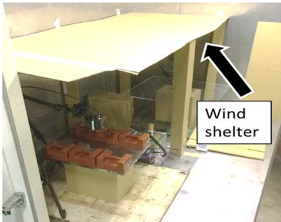
Fig.1 Equipment of Stacking Test
