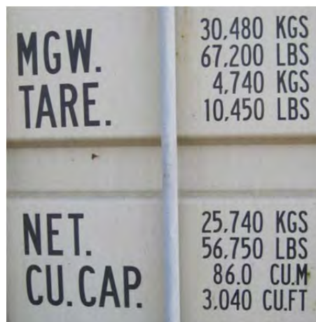
Fig.1 The ISO mark of a 45feet marine container photographed by the author.
