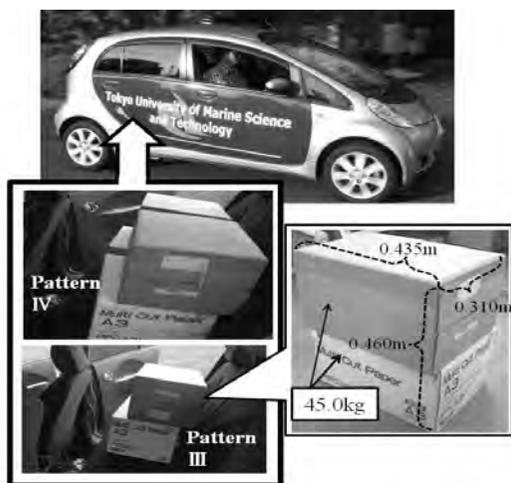
Fig.7 Conditions of cargoes on a moving automobile
