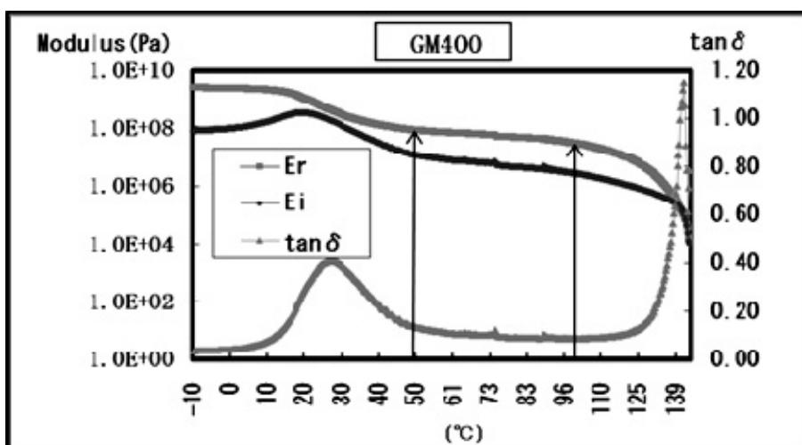
Fig.3 Storage elastic modulus at 50 and 100°C of GM400
