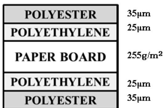
Fig.1 Structure of laminated board
