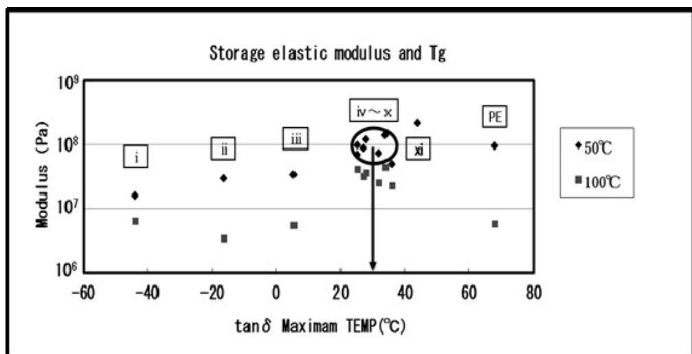
Fig.4 Plot of local maximal value of  $\tan\delta$  as  $T_g$  versus Modulus
