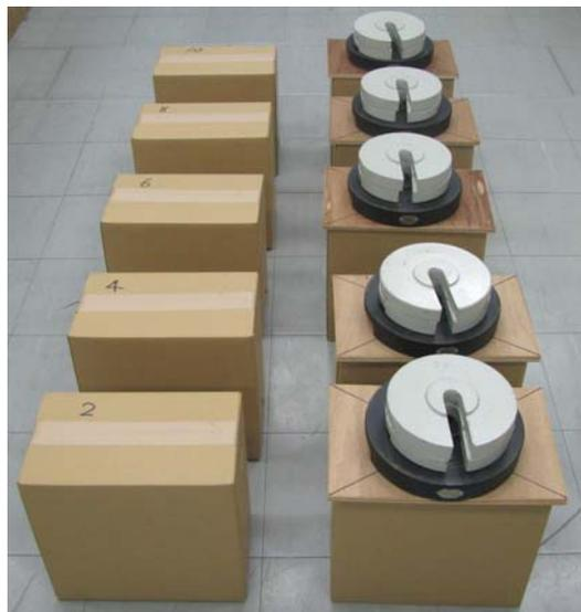
Fig.2 Load example of the static load.
