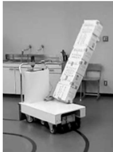
Fig.8 Rollover occurred on an experiment
