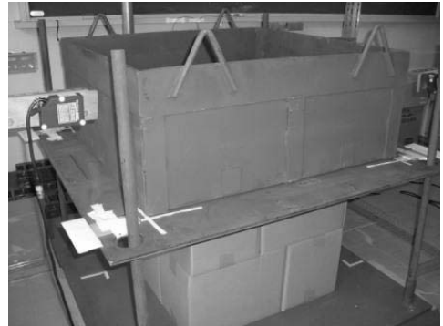
Fig.8 Stacking Test on 4c/s Pin-wheel Tier(2stairs)
