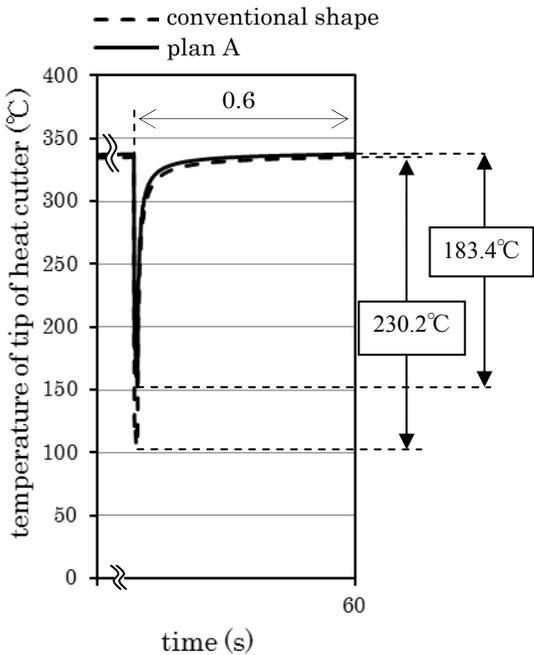
Fig.21 Temperature of a neighboring heat cutter tip after 60 s
