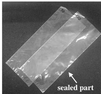
Fig.1 Example of a bag made using the side sealing production method
