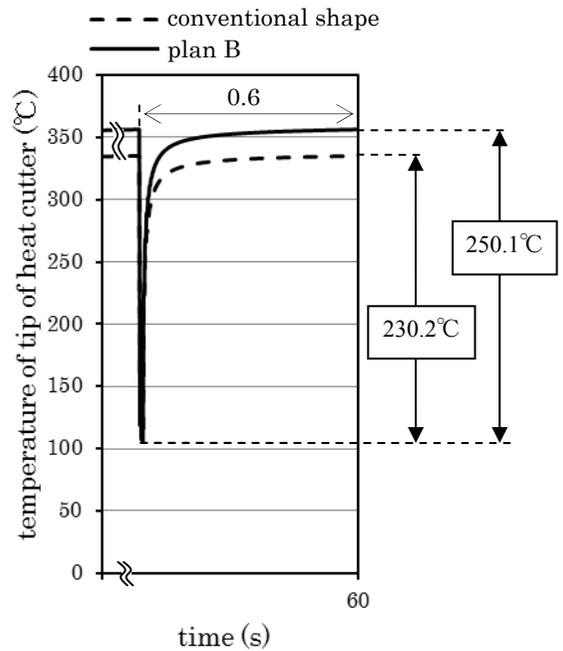
Fig.22 Temperature of a neighboring heat cutter tip after 60 s
