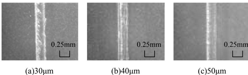
Fig.15 Seal thickness for each OPP film thickness
