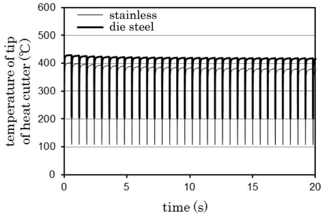
Fig.13 Temperature of tip of heat cutter (preset heater temperature 450°C)
