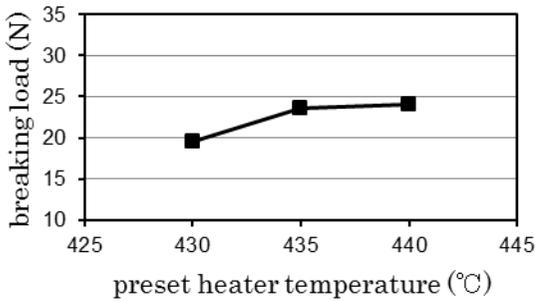
Fig.8 Relationship between breaking load and preset heater temperature (OPP film, thickness :30 $\mu$ m , number of shot :120shot/min)
