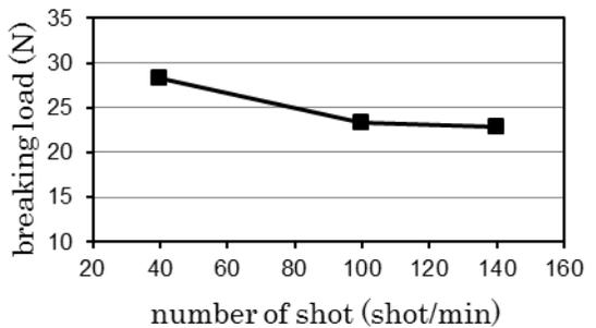
Fig.7 Relationship between breaking load and number of shot
