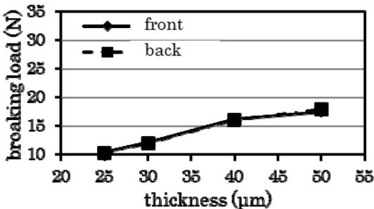
Fig.4 Relationship between breaking load and thickness in CPP film
