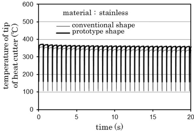
Fig.14 Transfer of heat in tip of heat cutter
