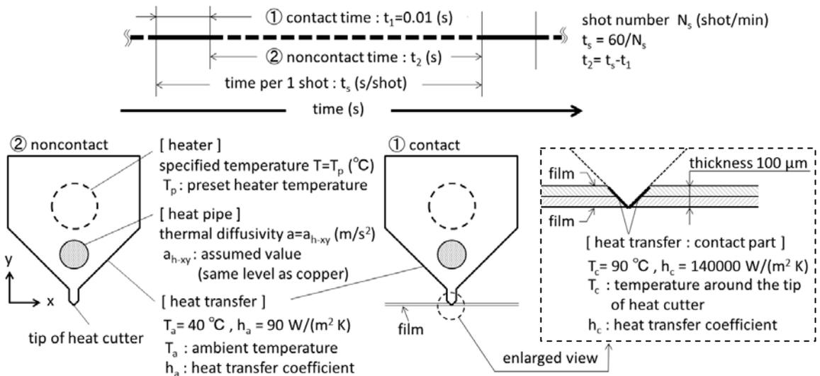
Fig.9 Analysis models and boundary conditions
