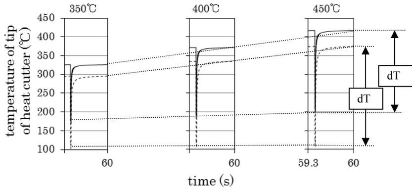
Fig.17 Temperature of a neighboring heat cutter tip after 60 s
