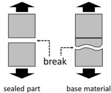
Fig.3 Schematic of break pattern
