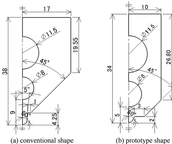
Fig.10 Shape and size of heat cutter (1/2 model) (units: mm)
