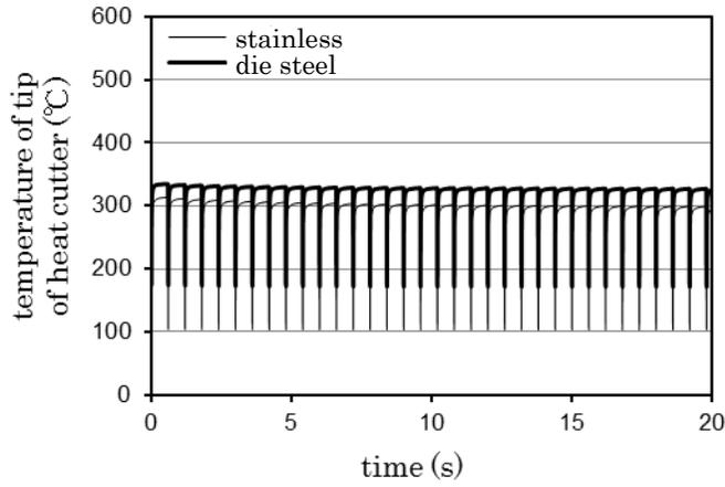
Fig.11 Temperature of tip of heat cutter (preset heater temperature 350°C)
