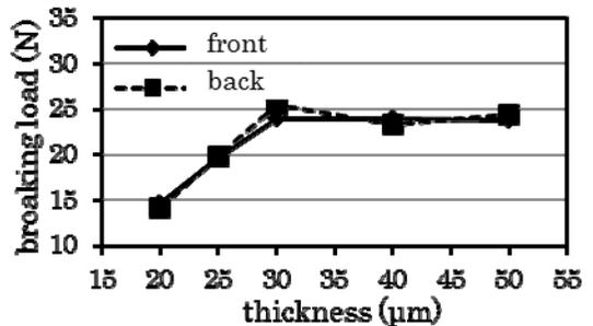
Fig.5 Relationship between breaking load and thickness in OPP film
