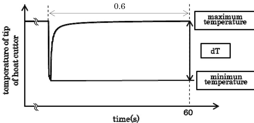
Fig.16 Method to determine maximum temperature, minimum temperature, and  $dT$
