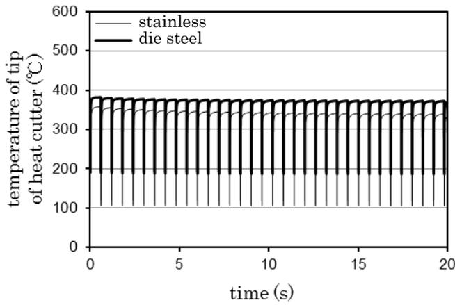
Fig.12 Temperature of tip of heat cutter (preset heater temperature 400°C)
