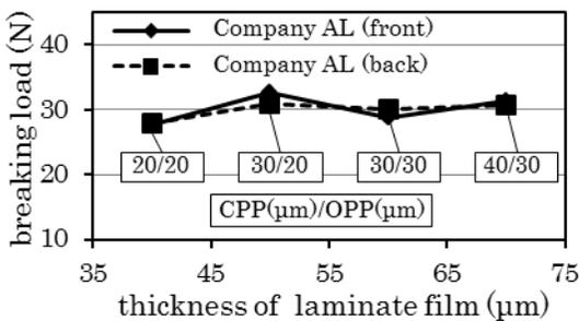
Fig.6 Relationship between breaking load and thickness in laminate film
