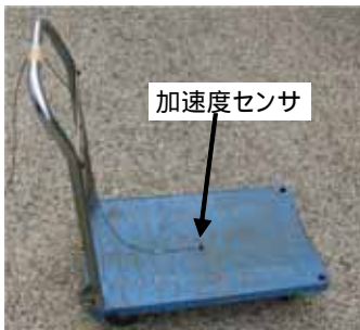
Fig.4 Position of acceleration sensor
