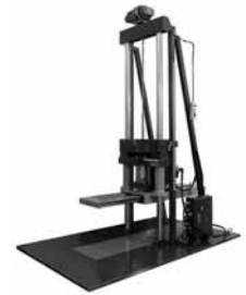
Fig.2 Slide type Free Fall Tester
